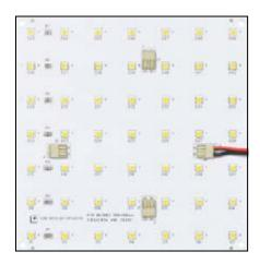
DC power can be supplied to the module at any of the Wago #2060 terminal blocks.
