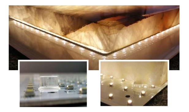
Optional half-inch Silicone bumpers can support heavy loads and offer protection to LED modules. Nine bumpers can support approximately 70-pounds per square foot.
