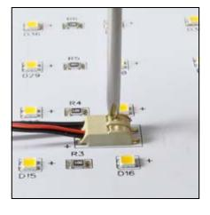
To release tension on the wire, gently press down, as shown. Too much pressure will damage the terminal block.
