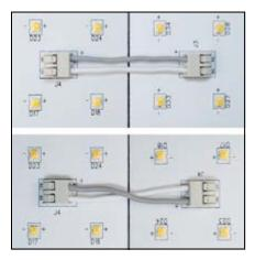
Modules are easily connected to each other with 18 AWG wire. Solid copper wire is easier to insert into the terminal block than stranded. Remove about 5/16-inch of the insulation and insert, as shown.
